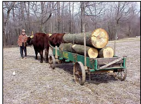
Figure 7. Steel-tired wagon for transporting logs. Steel tires create higher draft forces than pneumatic tires.
