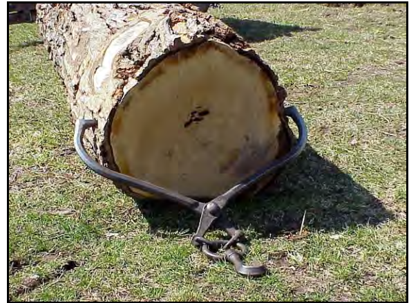
Figure 2. Logging tongs grasp the log for skidding.
