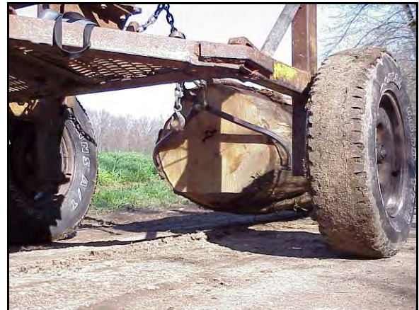
Figure 5. Chained short, a logging arch lifts the front of the log off the ground, keeping the log clean and reducing draft.
