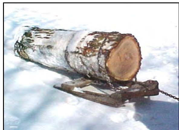
Figure 3. A go-devil elevates the hitch end of the log.
